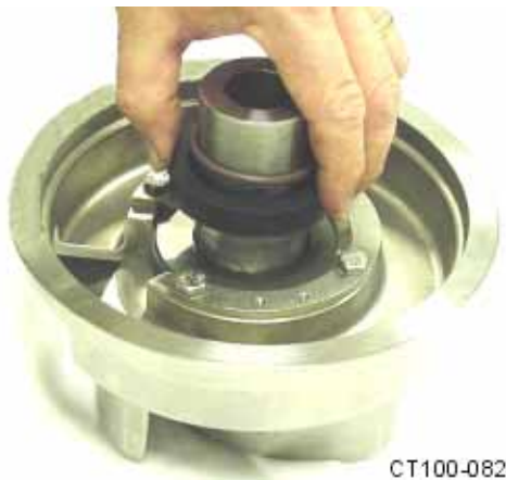
Figure 27 - Push Rotary Seal Down Until the O-ring is Released.
