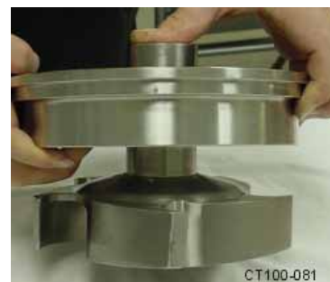
Figure 39 - Moving the Rotary Seal up the Shaft
